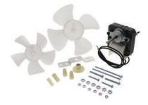
Part No. **M670 Motor (Utility)** 120V, 60 Hz, .55A, 3000RPM, 1-1/4" shaft Universal Replacement
