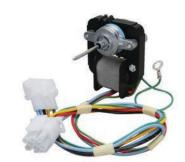
Part No. **241854301 Motor (Evaporator)** 120V, 60 Hz, .1A, 6W, 1-3/4" shaft Replacement for Electrolux
