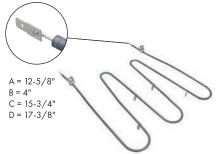
Part No. **B2200 Bake Element** Watts: 3500 Volts: 240 Has .250" male terminal push-in connection
