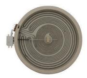
Part No. **WB30T10126** Surface Element (Radiant Heat) 11-3/4", 3000/1950/1050W@240V Replacement for GE
