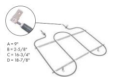
Part No. **B7340 Broil Element** Watts: 3400/2550 Volts: 240/208 Has .250" male terminal push-in connection COOKING
