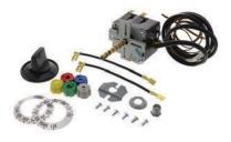
Part No. **6700S0011 Thermostat (Universal Electric)** 240V, 17 amp, 6 terminals Replaces most single or double pole thermostats
