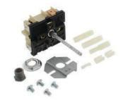
Part No. **5500202M** Infinite Switch Voltage sensing type, 240V, 13 amp Includes square breakoff shaft with multiple nylon adapter inserts for virtually all knobs used by Electrolux, GE, Maytag, Whirlpool & others
