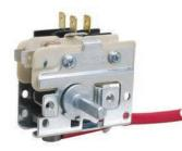
Part No. **74005019 Thermostat (Electric)** 240V, 27 amp, 8 terminals, Double pole Replacement for Whirlpool
