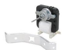
Part No. WR60X162 Motor (Evaporator) 120V, 60 Hz, .135A, 3000RPM, 1-5/8" shaft Replacement for GE
