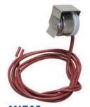
Part No. **MLT45 Defrost Thermostat** Open@45 Close@25 24" leads with stripped wire ends Universal Replacement
