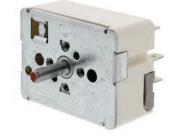
Part No. **7403P23960** Infinite Switch Current sensing type 240V, 8.9 - 11 amp Replacement for Whirlpool
