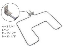
Part No. **B5002 Bake Element** Watts: 3000 Volts: 240 Has .250" male terminal push-in connection
