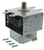
Part No. 10QBP0230 Magnetron 4.1 kV, 700-850 watts, Standard type, J Configuration, 30mm antenna
