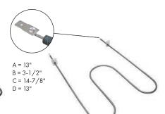
Part No. **B1551 Broil Element** Watts: 2100 Volts: 240 Has .250" male terminal push-in connection
