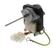
Part No. **WR60X 10172 Motor (Evaporator)** 115V, 60 Hz, .2A, 2800RPM, 2-5/8" shaft Replacement for GE
