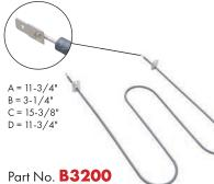
Broil Element Watts: 3000 Volts: 240 Has .250" male terminal push-in connection
