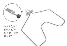
Part No. **WB44X10009 Bake Element** Watts: 2585/1940 Volts: 240/208 Has .250" male terminal push-in connection
