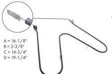
Part No. **B5103 Bake Element** Watts: 2600 Volts: 240 Has .250" male terminal push-in connection
