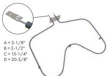
Part No. **B8541 Bake Element** Watts: 2400/1800 Volts: 240/208 Has .250" male terminal push-in connection
