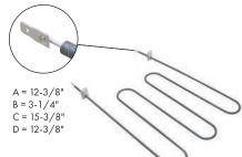
Part No. **B3301** Broil Element Watts: 4000 Volts: 240 Has .250" male terminal push-in connection
