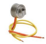
Part No. **WR50X 10025 Defrost Thermostat** L58-30F, 1/4" side push on clip 4-1/2" & 15-1/2" leads with stripped wire ends Replacement for GE
