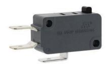
Part No. **28QBP0496 Switch (Button Type)** Universal Application SPDT NO/NC, 16 amps, 125/250V .320 x .250 terminal
