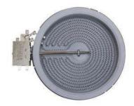
Part No. **RS65D12 Surface Element (Radiant Heat)** 6-1/2", 1200W@240V Replacement for Electrolux, Whirlpool
