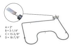
Part No. **B4107 Bake Element** Watts: 2585/1939 Volts: 240/208 Has .250" male terminal push-in connection
