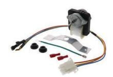
Part No. **61005935 Motor (Evaporator)** 120V, 60 Hz, .21A, 3000 RPM, 1-1/8" shaft Replacement for Whirlpool
