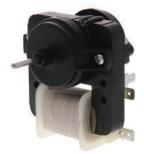
Part No. **W10189703 Motor (Evaporator)** 120V, 60 Hz, 135A, 3000RPM, 1" shaft Replacement for Whirlpool
