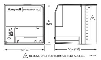
24 Vdc microprocessor-based integrated burner control for automatically fired gas, oil or combination fuel single burner applications. Provides level of safety, functional capability and features beyond the capacity of conventional controls.
