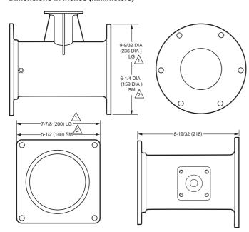
1 LG (LARGE) IS VENTURI MIXING UNIT VMU500 SM (SMALL) ARE VENTURI MIXING UNITS VMU150/300/335
