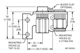
Non primary-aerated, insert orifice type pilot burner for main burner ignition. Used with Q309, Q340, and Q390 thermocouples or Q313 thermopiles.
