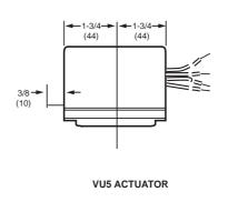
**VU53 AND VU54 VALVE WITH ACTUATOR**
