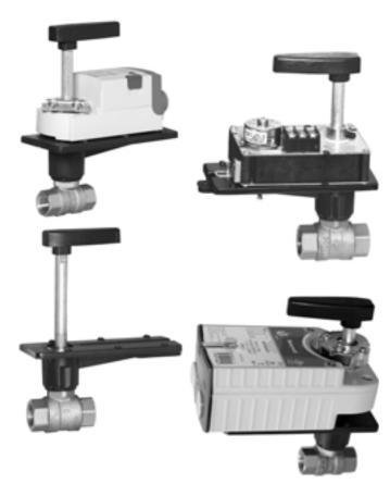
The VBN2 Two-Way Control Ball Valves control hot and chilled water with glycol solutions up to 50% in heating, ventilating, and air conditioning (HVAC) systems to provide two-position or modulating functions. These valve assemblies can be ordered with or without factory-mounted non-spring return or spring return direct-coupled actuators (DCA).
