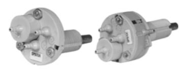
Used to manually position a remote damper actuator or to reset the setpoint of a pneumatic controller. They can also provide minimum damper position by setting a minimum pressure limit in the branch line to the damper actuator. Replacement kits are available for Johnson, Powers, Robertshaw, Barber-Colman, and older Honeywell switches.
