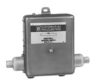
One-pipe, pressure operated device used to provide proportional control of pneumatic valve or damper actuators by varying the pressure to the actuators in relation to the pressure difference between two separate water pressures. Replacement devices are available for Johnson, Powers, Robertshaw, and older Honeywell pneumatic pressure controllers.
