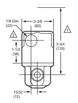
VU53 VALVE WITH VU448 ACTUATOR
