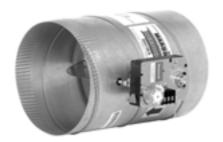
The Modulating Automatic Round Damper is a round damper with a 24-Vac, floating-control type modulating motor for bypass and zone damper control.
