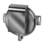
Dimensions, Approximate: 5.0 in. Diameter (127 mm Diameter) Electrical Ratings: 278 Va @ 24Vac; 300Va @ 120 to 277Vac Electrical Connections: #6-32 Screw terminal with cup washers Ambient Temperature Range: -40 F to +190 F (-40 C to +88 C)
