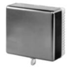
Inside Height: 5 1/16 in. (129 mm) Inside Width: 6 1/16 in. (154 mm) Outside Height: 6 1/2 in. (165 mm) Outside Width: 7 1/2 in. (191 mm) The Versaguard® Universal Thermostat Guards cover wall thermostats and protect against tampering, damage and unauthorized adjustment of thermostat settings.
