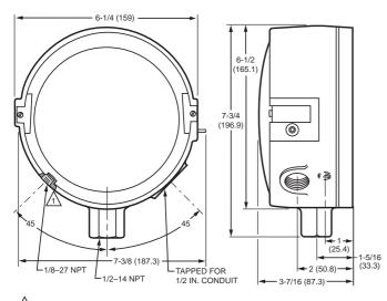
VENT TAPPING. REMOVE DUST-SEAL LABEL BEFORE MOUNTING.
