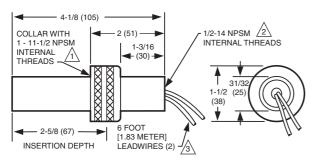
1\ DIN APPROVED C7035A1064 HAS 1-11 BSP.P1 INTERNAL MOUNTING THREADS. DIN APPROVED C7035A1064 HAS 1/2-14 BSP-F INTERNAL MOUNTING THREADS.
