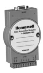
The QM4520A RS-232 to RS485 Converter allows a PC to communicate with multiple devices on a single bus, over greater distances.
