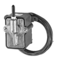
One-pipe, direct-acting temperature sensor used with RP908/RP920 Controllers to provide proportional control of pneumatic valve or damper actuators. Averaging, liquid-filled element for duct mounting.
