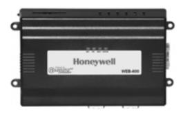
The WEB-600 is ideal for smaller facilities, remote sites, and for distributing control and monitoring throughout large facilities. Optional I/O modules can be plugged in for applications where local control is required. The WEB-600 controller also supports a wide range of field busses for connection to remote I/O and standalone controllers. In small facility applications, the WEB-600 controller is all you need for a complete system.
