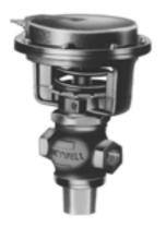
Two-position, three-way, pneumatic air valve used to control main airflow in large Day-Nite or Summer-Winter pneumatic control systems. Replacement device is available for Johnson, Powers, Robertshaw, Barber-Colman, and older Honeywell devices.
