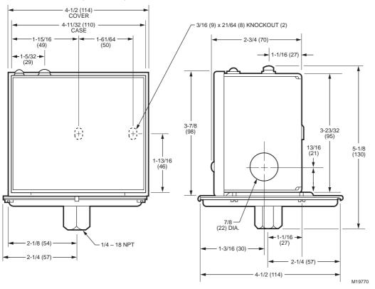
Application: Provide operating control and automatic limit protection for pressure systems with pressures up to 4 psi (8 kPa)
