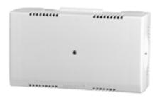
The Excel 15 W7760A Building Manager is a LonMark® compliant device that can be used to monitor and control HVAC equipment and other miscellaneous loads in a distributed network. The optional lithium battery (not included, purchased locally) allows continuous power so trend logs and alarms can be maintained for up to four continuous years. The W7760A Building Manager
