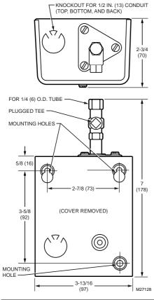
Used to convert a pneumatic signal from a controller to an electrical switching action to provide start and stop control of equipment such as fans and pumps. Replacement devices available for Johnson, Powers, Robertshaw, Barber-Colman, and older Honeywell pneumatic/electric switches. Adjustable setpoint.
