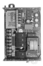
The L7224U Oil Electronic Aquastat® Controller provides electronic temperature sensing in a UL limit-rated controller with a single sensing probe. The L7224U controls the circulator, oil burner and boiler temperature. The L7224U replaces the L8124A, L8124C, L7124U, L7148A, L7248A,C, L7224A,C, and L8148A Controllers. The Aquastat Controller is intended for use in residential-type applications. The L7224U provides status and
