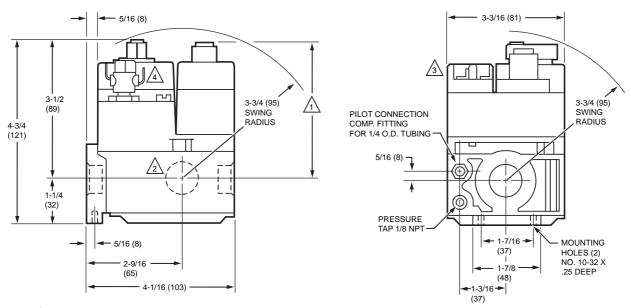
WITH V5306 (ILLUSTRATED), V5307 OR 5390 PRESSURE REGULATOR: 24V MODELS-3-1/2 (89), 120V MODEL-3-5/8 (92) MANUAL MODELS-2-13/16 (71), FOR V5308 ADD 5/8 (16) TO DIMENSIONS GIVEN.
