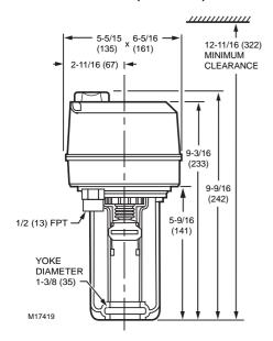
Actuator Type: Valve Fail Safe Mode: Stays in place (Rated) Stem Force: 135 bf (600 N)
