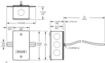
DEPENDING ON THE MODEL, THE ELEMENT LENGTH IS EITHER 12 FT (366 CM) OR 24 FT (732 CM).
