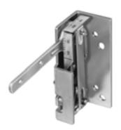
One-pipe, single temperature, low-capacity pneumatic thermostat used to provide proportional control of pneumatic valves and mixing boxes in heating and air conditioning systems. It mounts in a slot or light troffer diffuser or a return air grill.
