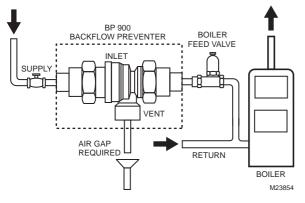
The BP900 is a double check backflow preventer with an intermediate vacuum breaker designed to prevent the backflow of contaminated water into the potable water supply. Designed for the use on small supply lines, it protects against both backflow and back siphonage for continuous pressure applications.
