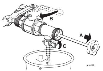
Unscrew end cap and remove cartridge from chamber. Clean or replace cartridge.
