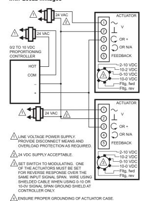
Wiring of tandem floating actuators with Q5022 linkages
