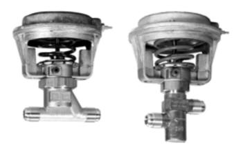
Single-seated, straight-through, pneumatic valves used for proportional control of unit air conditioners using hot and/or chilled water. Replacement devices are available for Johnson, Powers, Robertshaw, Barber-Colman, and older Honeywell
