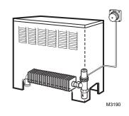
Capacity: Standard Materials (Body): Nickel Plated Bronze Differential Pressure Rating: With T100 or T200: 15 psi (103 kPa) For low noise: 3 psi (20 kPa) Pressure Ratings (Hot Water): 150 psi maximum (1034 kPa)
