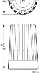
**Application:** High Capacity Thermostatic Radiator Actuator **Used With Valve:** V110
