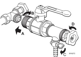
Open shut-off on drain cock, removing excess water and steam from chamber.
