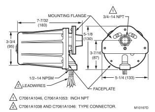
**Description:** Dynamic Self-checking Ultraviolet Flame Detector
