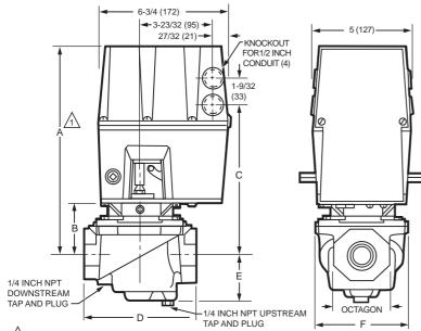
ALLOW 2 IN. (51 mm) CLEARANCE FOR ACTUATOR REMOVAL.
