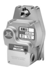
The ML8135 Fast-Acting, Two-Position Actuators are spring return direct coupled actuators (DCA) with an integral junction box for on/off damper control.
