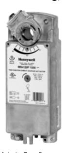
The MS8120F,S is a 175 lb-in (20Nm), spring return direct-coupled, 24 Vac actuator that accepts two position (SPST) control with an integral junction box. The actuator accepts an on/off signal from a single-pole, single-throw (SPST) controller. They are designed to operate reliably in smoke control systems requiring Underwriter's Laboratories Inc. UL555S ratings up to 350 F.
