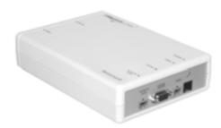
The Excel 10 Q7770A RapidLink device is a complete network interface unit for a FTT LonWorks® Bus network. RapidLink is equipped with an on-board modem that eliminates the requirement
