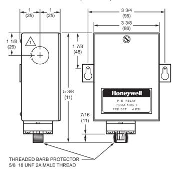
KNOCKOUT ON ONE SIDE FOR 3/4 1NCH CONDUIT. KNOCKOUTS ON OPPOSITE SIDE, TOP, AND BACK FOR 1/2 INCH CONDUIT.
