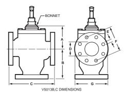
VALVE SIZE IN INCHES (MM) 2-1/2 (DN65) 3 (DN80) 4 (DN100) 5 (DN125) 6 (DN150) Α 5-1/4 (133) 4-1/2 (114) 6-1/4 (159) 7-1/4 (184) 5-7/8 (149) 6-7/17 (164) 6-5/8 (168) 8-11/16 9-5/8 (244) 10-11/16 (271)9-1/2 (241) 16-1/2 (419) С 11 (279) 13 (330) 15 (381) D 3 (76) 4 (102) 5 (127) 6 (152) 3/4 (19) Е 3/4 (19) 3/4 (19) 7/8 (22) 7/8 (22) 5-1/2 (140) 7-1/2 (191) 9-1/2 (241) F 6 (152) 8-1/2 (216) 7-1/2 G 7 (178) 11 (279)
