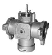
The V5197A is a firing rate valve used to provide variable flow control of air, natural gas, liquefied petroleum (LP), and manufactured gases. The V5197A is actuated by a ML7999A or B firing rate motor that can be mounted directly on the valve. The V5197A is not applicable as a safety shutoff valve. The V5197A is specially designed to provide fine control of gas flow in
