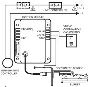
POWER SUPPLY. PROVIDE DISCONNECT MEANS AND OVERLOAD PROTECTION AS REQUIRED.
