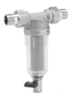
Materials (Body): Dezincification-resistant (DZR) forged Brass Connection Type: NPT External Threaded and Sweat Sump: Clear Plastic
