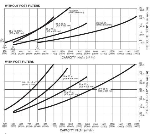
MINIMUM RECOMMENDED cfm FOR 20 x 12-1/2 in. (508 x 318 mm) MODEL.
