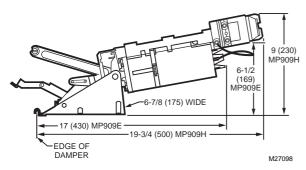
Actuator Type: Damper Actuator Force: Medium Fail Safe Mode: Spring Return
