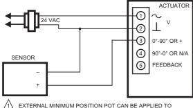
EXTERNAL MINIMUM POSITION POT CAN BE APPLIED TO TERMINAL 4 90°-0°. M2951
