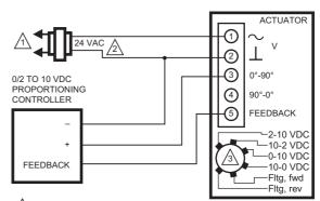
LINE VOLTAGE POWER SUPPLY. PROVIDE DISCONNECT MEANS AND OVERLOAD PROTECTION AS REQUIRED.
