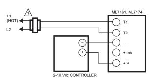
POWER SUPPLY. PROVIDE DISCONNECT MEANS AND OVERLOAD PROTECTION AS REQUIRED.
