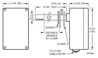
The H7015B Combined Humidity/Temperature Duct Sensor combines a capacitance-type relative humidity sensor with a PT1000 or BALCO 500 temperature sensor in one housing. These sensors can be used for discharge, outside or return air control or as a high-limit sensor in applications such as steam humidification.
