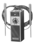
Operating controller for a hot water or warm air heating system. Used for line voltage, low voltage or millivolt (Powerpile) switching. Maintains proper balance between heating medium temperature and outdoor temperature.
