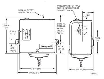
**Type:** Averaging element **Voltage:** 120 Vac; 240 Vac **Frequency:** 50 Hz; 60 Hz
