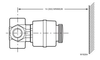
Torque Rating: 60 lb-in. Manual declutch (7 Nm Manual declutch)
