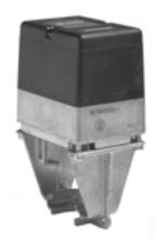
Actuator Type: Valve Fail Safe Mode: Stays in place (Rated) Stem Force: 160 bf (710 N) Cable Entry: 7/8 in. hole for 1/2 in. conduit
