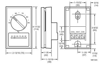
Application: T451-Heating; T651-Heating and cooling
