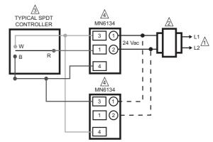
A POWER SUPPLY PROVIDES OVERLOAD PROTECTION AND DISCONNECT MEANS.
