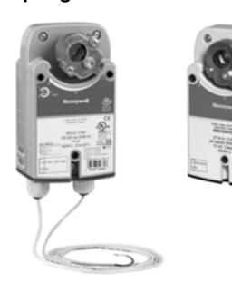
The MS8105 is a 44 lb-in (5Nm), spring return direct-coupled, line voltage actuator that accepts two-position (SPST) control for: air dampers, air handlers, ventilation flaps, louvers, and ball valves.
