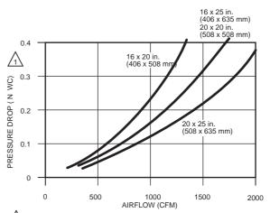
WHEN FIRST INSTALLED. PRESSURE DROP INCREASES AS FILTER
