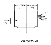
VU53 AND VU54 VALVE WITH ACTUATOR
