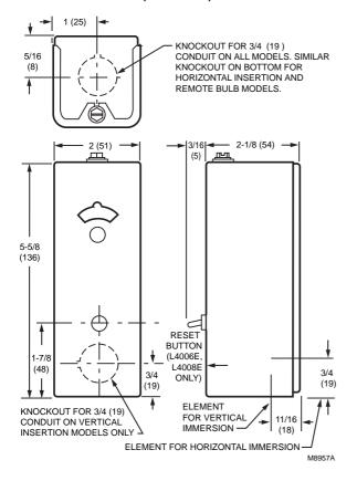
Aquastat® Controllers are immersion type devices for limiting or regulating the temperature of liquids in boilers, storage tanks, and other applications where temperature control is required.
