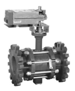
50% in closed loop heating, ventilating, and air conditioning (HVAC) systems to provide two-position or modulating functions. These valve assemblies can be ordered with or without factory-mounted non-spring return or spring return direct-coupled actuators (DCA). Sizes from 4 to 6 inch with ANSI Class 125 flanged connections
