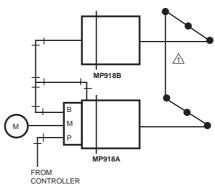
SECTIONS OF LARGE DAMPER REQUIRING MORE THAN ONE OPERATOR MUST BE LINKED
