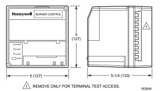
Microprocessor-based integrated flame switch for detecting a flame using rectification, ultraviolet (UV) or infrared (IR) source. Provides level of safety, functional capability and features beyond conventional controls.
