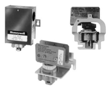
Pneumatic-electric switches (P658A,B,E and F) used to convert a pneumatic signal from a controller to an electrical switching action (SPDT) to provide start and stop control of equipment such as fans and pumps. Replacement devices available for Johnson, Powers, Robertshaw, Barber-Colman, and older Honeywell pneumatic/electric
