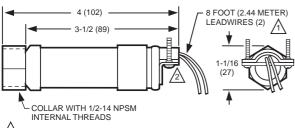
C7027A1064 HAS 24 FOOT (7.32 METER) LEADWIRES. C7027A1114 HAS 44 IN. (1.118 M) LEADWIRES WITH 22 IN. (558 MM) FLEXIBLE CONDUIT.
