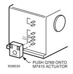
Q769 Adapter is used to provide a modulating signal to the M7415 Economizer Damper Motors when used with a controller.
