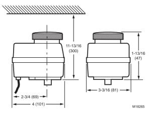
Aux Switch Ratings: 24 Vac, 3A, 24 VA pilot duty, Class 2, normally closed, Gray cable. S1 (black/gray pair) opens at left (CCW) end stop. S2 (brown/pink pair) opens at right (CW) end stop.
