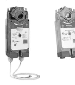
Actuator Type: Damper; Valve Rotational Stroke: 95 ±3 degrees Fail Safe Mode: Spring Return Torque Rating: 88 lb-in. (10 Nm) Spring Return Torque: 88 lb-in. (10 Nm) Spring Return Direction: By orientation
