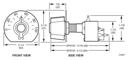
Air Connections: Barb fitting for 5/32 in. (4 mm) O.D. plastic tubing
