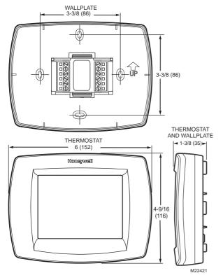
The TB8220 provides temperature control for gas, oil, electric and heat pumps for up to 2 heat, 2 cool systems.
