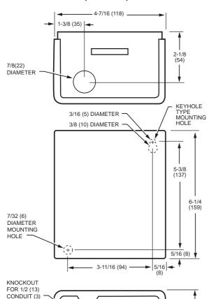
The R8845U Universal Switching Relay with 24 V transformer provides intermediate switching of line-and low-voltage devices from a line- or low-voltage controller and is typically applied in Hydronic heating systems.
