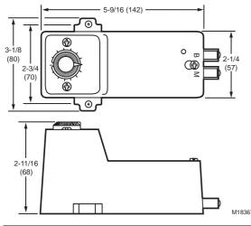
Two-pipe, single temperature, pneumatic temperature controller used to provide proportional control of pneumatic valves and damper actuators in heating and air conditioning systems. Replacement devices are available for Johnson, Powers, Robertshaw, Barber-Colman, and older Honeywell two-pipe pneumatic temperature controller.
