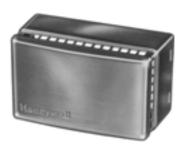
One- or two-pipe direct-acting temperature sensor used with RP908/RP920 Controllers to provide proportional control of pneumatic valve and damper actuators.
