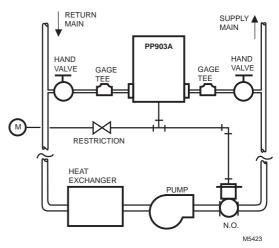
**Application Type:** Differential Pressure **Action:** Reverse Acting, Direct Acting
