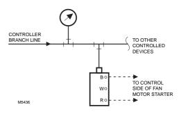
Air Connections: Compression fitting 1/4 in. (6 mm) O.D. tubing Current: 120 Vac: 8.0 AFL, 48.0 LRA, 17.0 A resistive; 208/240 Vac: 5.1 AFL, 30.6 ALR, 17.0 A resistive; 270 Vac: 17.0 A resistive; 480
