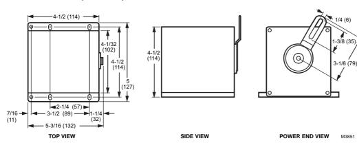
Fail Safe Mode: Spring Return Torque Rating: 25 lb-in. (2.8 Nm)
