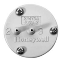
Three-port relays used in HVAC systems to perform a variety of relay functions; transmit the higher of two input signals, lock out one pressure signal when a second signal is higher, or transmit the lower of two pressure signals. Replacement devices are available for Johnson, Powers, Robertshaw, Barber-Colman, and older Honeywell devices.
