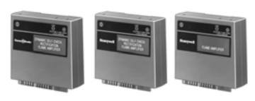
Solid state plug-in amplifiers that respond to flame detector inputs to indicate the presence of flame when used with 7800 SERIES relay modules.
