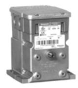
Series 72 Modutrol IV Motors are spring return and non-spring return motors (per motor type) used to control dampers and valves. The motors accept a current or voltage signal from an electronic controller to position a damper or valve at any point between open and closed.
