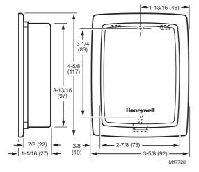
The T7047 Electronic Thermostats, Remote Space Sensors are used with T7300 thermostats and W973 controller to provide modulating space temperature control.
