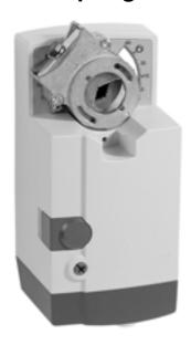
The MN7220 is a 175 lb-in (20Nm), non-spring return, direct-coupled, low voltage actuator that accepts adjustable modulating (0/2-10 Vdc) control for: air dampers, air handling units, ventilation flaps, louvers, and ball valves.
