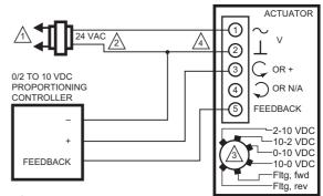
LINE VOLTAGE POWER SUPPLY. PROVIDE DISCONNECT MEANS AND OVERLOAD PROTECTION AS REQUIRED.
