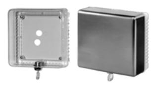
Inside Height: 4 7/16 in. (113 mm) Inside Width: 4 7/16 in. (113 mm) Outside Height: 5 7/8 in. (149 mm) Outside Width: 5 7/8 in. (149 mm) The Versaguard® Universal Thermostat Guards cover wall thermostats and protect against tampering, damage and unauthorized adjustment of thermostat settings.
