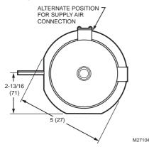
Actuator Type: Damper Actuator Force: Medium Fail Safe Mode: Spring Return Air Connections: 1/8 in. NPT
