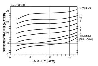
Maximum Inlet Pressure Rating (psi): 85 Psi Outlet Pressure Adjustment Range (psi): 0-17 psi Pipe Connection: Angle type, female threaded NPT
