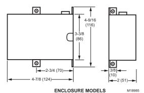
The Q7002 Interface Modules allow controllers with an otherwise incompatible signal to control an Economizer Logic Module or Direct Coupled Actuator.
