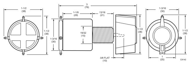
Air Connections: Barb fitting for 5/32 in. (4 mm) O.D. plastic tubing Airflow Usage: 0.175 scfm (82.6 mL/s) minimum at 1 psi pressure drop
