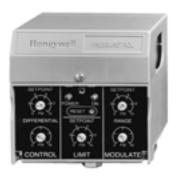
Line voltage pressure controller that provides automatic operating control, automatic limit protection, manual reset limit protection, and 4-20ma modulating firing rate control for pressure systems up to 300 psi.
