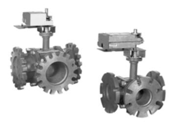
The VBF3 Three-Way Ball Valve Assemblies, with and without actuators, control hot and chilled water with glycol solutions up to 50% in closed loop heating, ventilating, and air conditioning (HVAC) systems to provide two-position or modulating functions. These valve assemblies can be ordered with or without factory-mounted non-spring return or spring return direct-coupled actuators (DCA).
