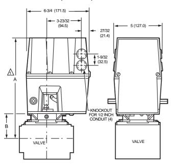
ALLOW 4 IN. (101.6 MM) CLEARANCE FOR ACTUATOR REMOVAL.
