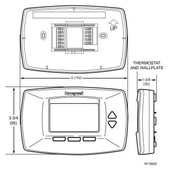
The TB7220 provides temperature control for gas, oil, electric and heat pumps for up to 2 heat, 2 cool systems.
