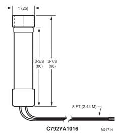
The Solid State Ultraviolet Flame Detectors detect the ultraviolet radiation emitted by combustion flames. The flame detectors are used with Honeywell flame safeguard controls to provide flame supervision for gas, oil, or combination gas-oil burners.
