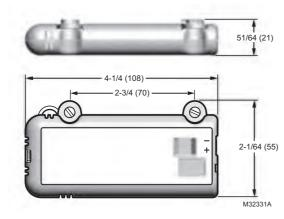
The C7600A,C Solid State Humidity Sensors sense relative humidity in air and are used with controllers that can process a 4 to 20 mA signal.
