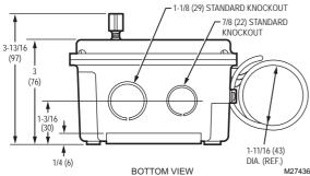
Provide line voltage control of heating, cooling and ventilating systems in farm buildings, storage areas and industrial environments; watertight, dust-proof enclosure.
