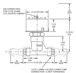
ALLOW 1-1/2 IN. (38 MM) MINIMUM CLEARANCE TO SERVICE VALVE. 2-1/2 IN. (63 MM) CLEARANCE TO CONNECT TUBING STRAIGHT TO CONNECTOR. IF CLEARANCE IS LESS THAN 2-1/2 IN. (63 MM), USE AN ELBOW CONNECTOR
