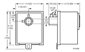
ML7999B Universal Direct Coupled Actuator provides 100 lb-in. torque, 4 to 20 mA control input to control combustion air dampers and modulation valves. The actuator includes precision drive shaft control and integral power supply capable of direct line voltage connection.
