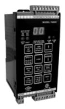
The 700 is a signal processor which amplifies and conditions the viewing head signal for use with a burner management system. It provides a 0/4-20mA output signal, two SPDT flame relay outputs and one SPDT self-check relay output.
