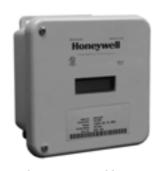
The H50 Series Class 500 Meter is a 3-element meter with communications. The device is used to monitor electric power usage of individual loads after the utility meter and store kW and kVAR data for automatic meter reading. Installation must only be performed by qualified personnel and in accordance with these instructions and all applicable local and national electrical codes.
