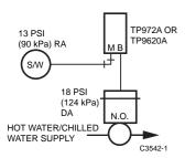
Application Type: Wall Thermostat, Heat/Cool Operation
