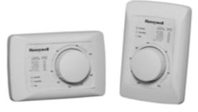
The H8908A Humidistat and H8908D Dehumidistat (humidity controllers) provide automatic low voltage control of humidifiers and dehumidifiers or ventilators, respectively, in central heating and air conditioning systems. They have a SPST, snap-acting, dust-proof switch and are designed for wall or surface duct mounting.
