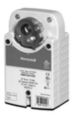
Actuator Type: Damper; Valve Rotational Stroke: 95 ±3 degrees Fail Safe Mode: Spring Return Torque Rating: 27 lb-in. (3 Nm) Spring Return Torque: 27 lb-in (3 Nm) Spring Return Direction: By orientation
