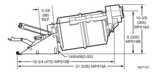
Used for proportional control of medium- to large-size dampers in HVAC systems. The MP918A,B are rolling diaphragm, piston-type actuators. The MP918A has a positive positioner. Replacement devices are available for Johnson, Powers, Robertshaw, Barber-Colman, and older Honeywell actuator models.
