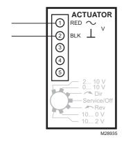
Cable writing for floating and modulating (0/2-10 Vdc) control, MS7505W series.
