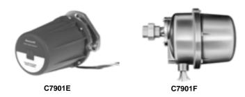
A self-checking flame detector using a solid state UV sensor to detect ultraviolet radiation in flames for supervision of gas, oil or combination gas-oil burners.
