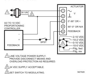
Cable wiring for low voltage, two-position control, MS8105W series
