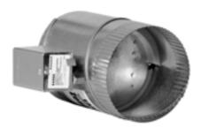
The EARD is a round damper with a 24 Vac powered-open/springclosed motor. It is used for fresh air intake for ventilation or for combustion makeup air.
