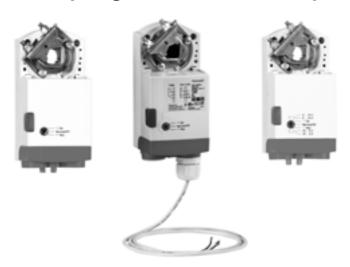
The MN7505W is a 44 lb-in (5Nm), non-spring return, direct-coupled, low voltage actuator that accepts adjustable modulating (0/2-10 Vdc) or on/off (SPDT) control for: air dampers, air handling units, ventilation flaps, louvers, and ball valves. This model includes a 3 foot whip.
