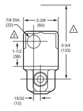
**VU53 VALVE WITH VU448 ACTUATOR**
