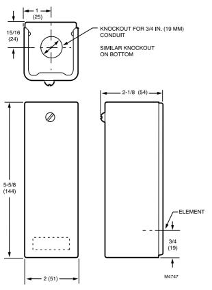
L8100A,B, and C are immersion type controllers for regulating and limiting the tank temperature in water heaters. As the water temperature rises past the setpoint, the controller switches off the gas valve.
