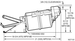
Actuator with Internal N.O. Trunnion Mounting Bracket
