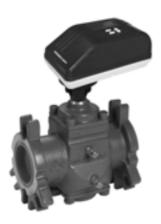
The VRW2 two-way dynamic pressure-regulating control valves maintain constant flow of hot and chilled water in closed-loop heating, ventilating, and air conditioning (HVAC) systems regardless of head pressure fluctuations above minimum specified pressure drop. These valves come complete with proportional, stay-in-place or electronic fail-safe actuators.
