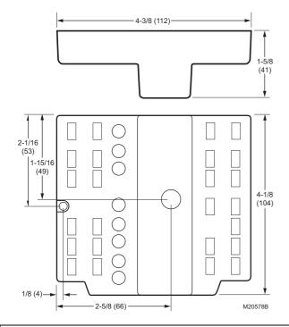
W7212, W7213, and W7214 Economizer Logic Modules are used with CO2 Demand Control Ventilation (DCV) Sensors, and solid state C7400A Enthalpy Sensors or C7660 Dry Bulb Temperature Sensors. All models proportion outdoor and return air dampers for control of free cooling in commercial HVAC equipment.
