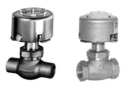
Normally-open, single-seated valve provides proportional control of steam or hot or cold water in terminal units. Replacement devices are available for Johnson, Powers, Robertshaw, Barber-Colman, and older Honeywell devices.
