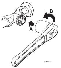
Tighten Cartridge Changer to valve body and close off drain cock.
