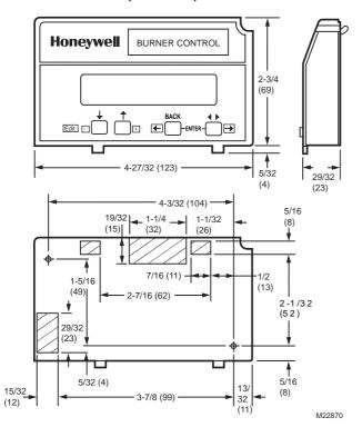
Provides current status of burner sequence, timing information, hold information and lockout information, as well as selectable or preemptive messages.
