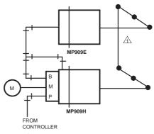
SECTIONS OF LARGE DAMPER REQUIRING MORE THAN ONE OPERATOR MUST BE LINKED
