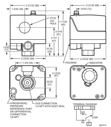
Application: Safety devices used in positive-pressure or differentialpressure systems to sense gas or air pressure changes
