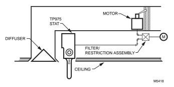
Application Type: Single temperature, low capacity, pneumatic
